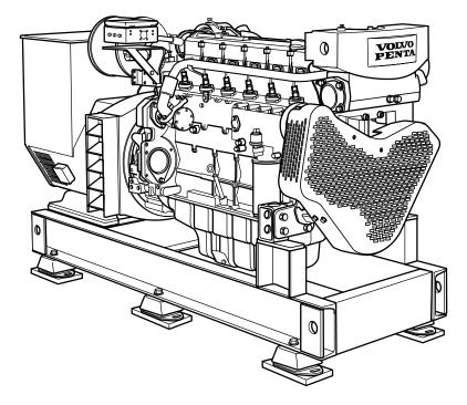
Easily accessible maintenance points and single side servicing contribute to the ease of servicing the engine. Liners of wet and replaceable type, inclined connecting rod caps and replaceable valve seats make even major maintenance possible to carry out on-board.
